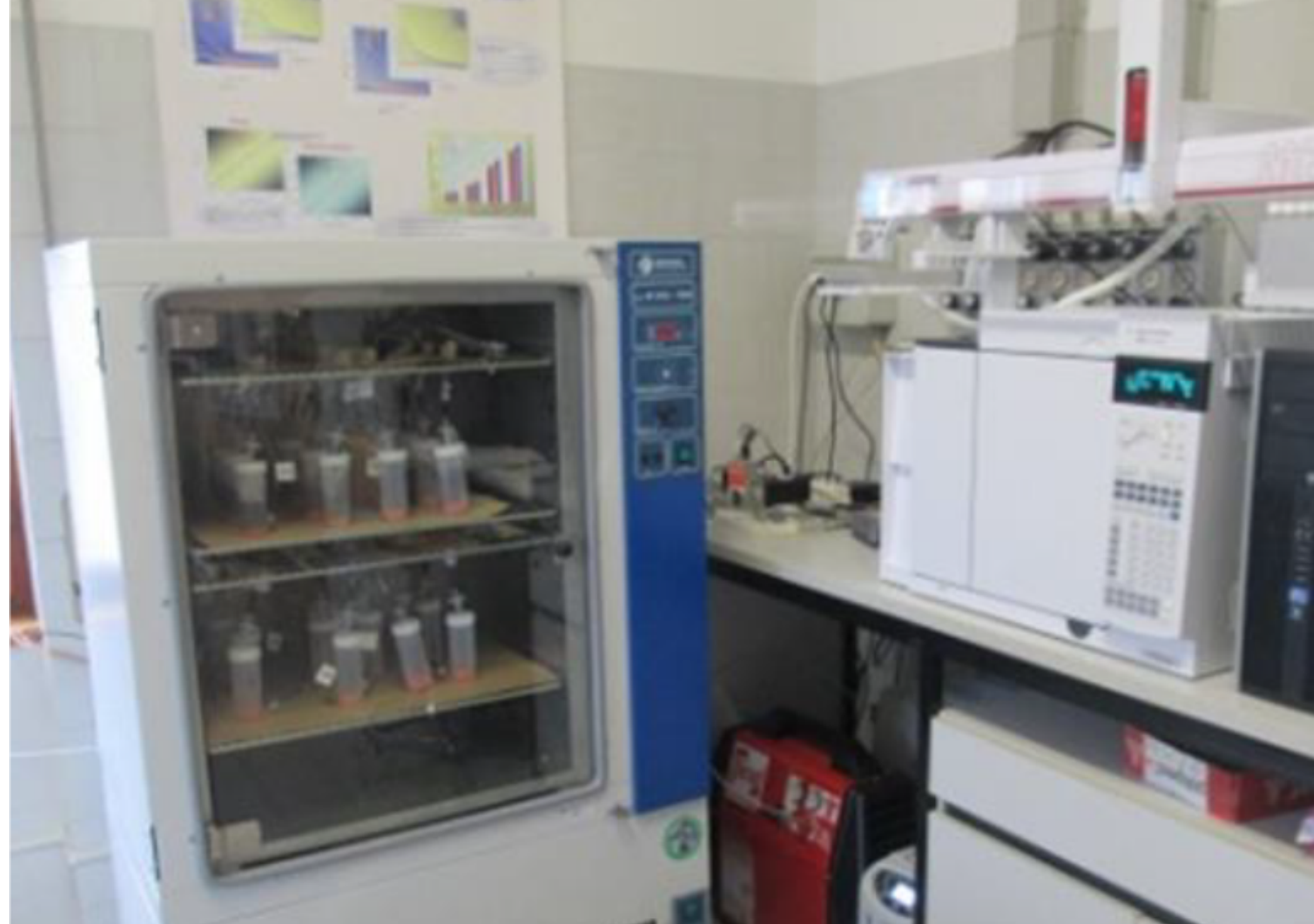
Figure 1. Automated gas chromatography system for GHG analyses of amended soils incubated in laboratory.
